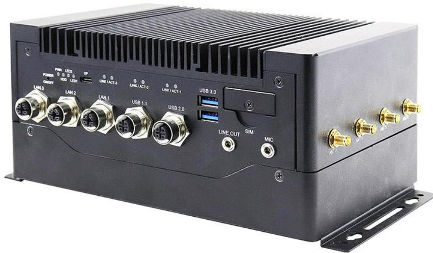
The oblique view also shows four (4) antenna connectors on the right side.
